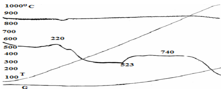
Fig. 2. DTA/TG curves of the “Uvgundatsan” iron ore.
